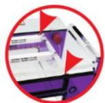
RapidCast™ Technolgy uses trays with incorporated end gaskets, to easily cast gels in the gel unit base Turn tray across gel platform to seal and pour Align with platform to run No tape! No Leaks! Fast & Efficient
